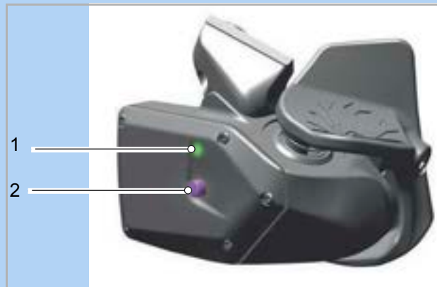
Figure 107: Rear derailleur SRAM AXS Controller with LED indicator (rear derailleur) (1) and AXS button (rear derailleur) (2)
