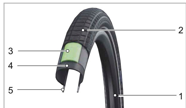
Figure 30: Structure of tube-type tyre
