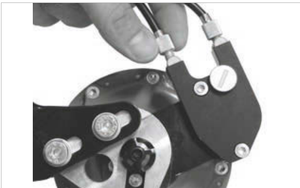
Figure 240: The tension adjuster on ROHLOFF hub versions with external switch control is located on the cable box positioned on the left-hand side
