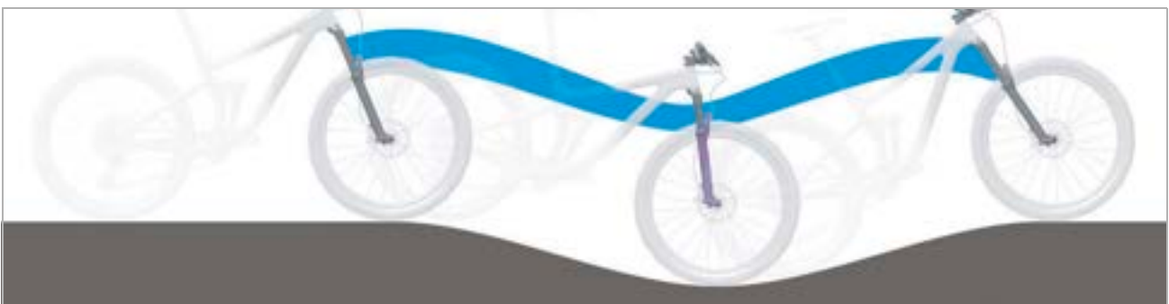
Figure 22: Optimum suspension fork ride performance on hilly terrain
