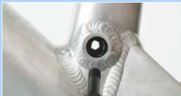
Figure 306: Hole in the Postpin interface
