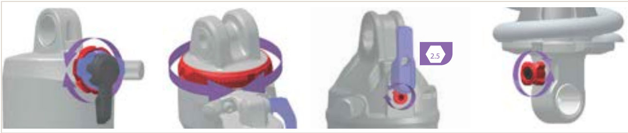
Figure 176: The position and shape of the rebound adjuster (rear frame damper) depends on the model. Rebound adjusters are always red
