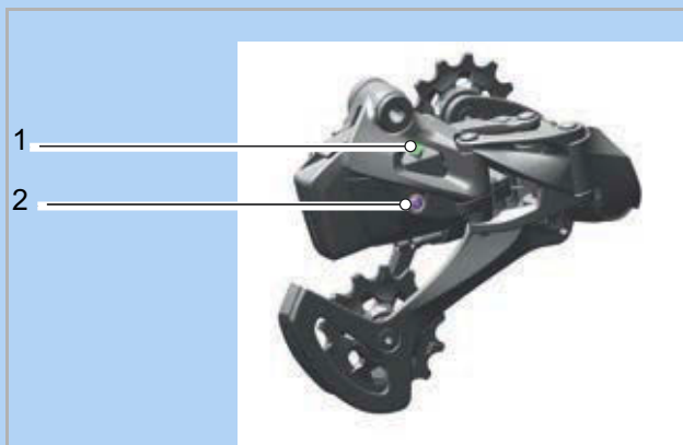
Figure 106: SRAM XX1 EAGLE AXS rear derailleur with LED indicator (rear derailleur) (1) and AXS button (rear derailleur) (2)
