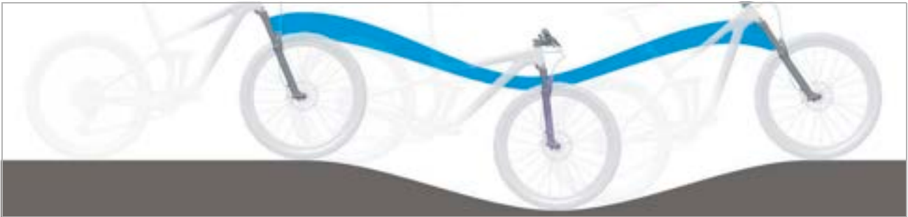
Figure 321: Excessively soft suspension in the suspension fork on hilly terrain
