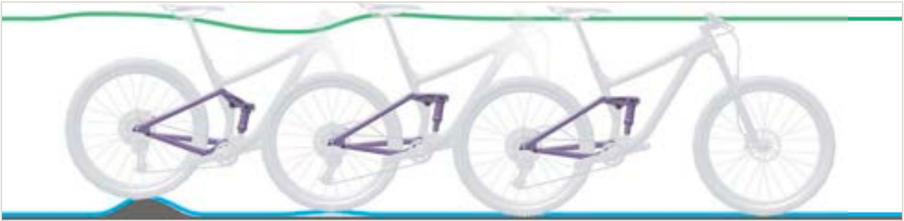
Figure 323: Rear frame damper rebounding too quickly
