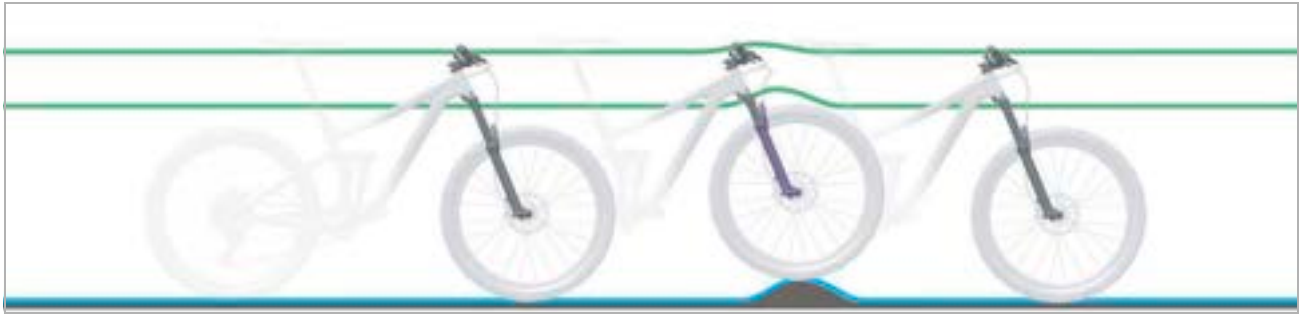
Figure 23: Optimum suspension fork ride performance over bumps
