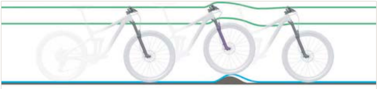
Figure 315: Excessively hard damping in the suspension fork on bumps
