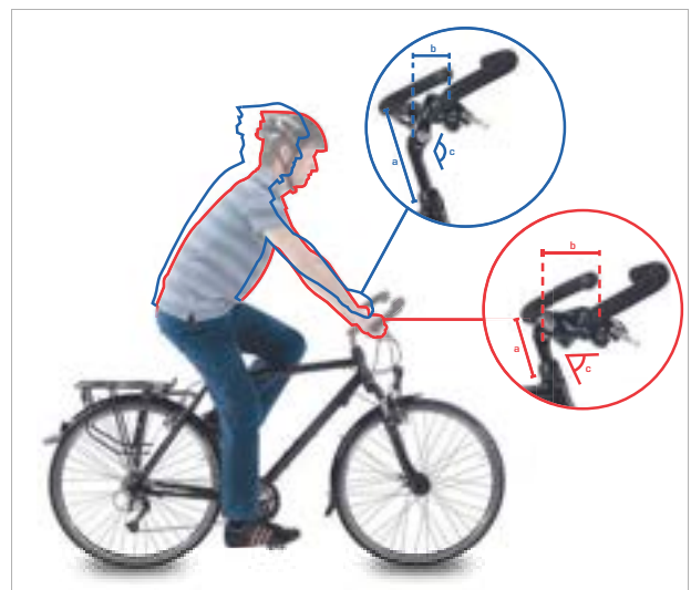
Figure 141: City bike (blue) and trekking bike position (red) by changing the angle
