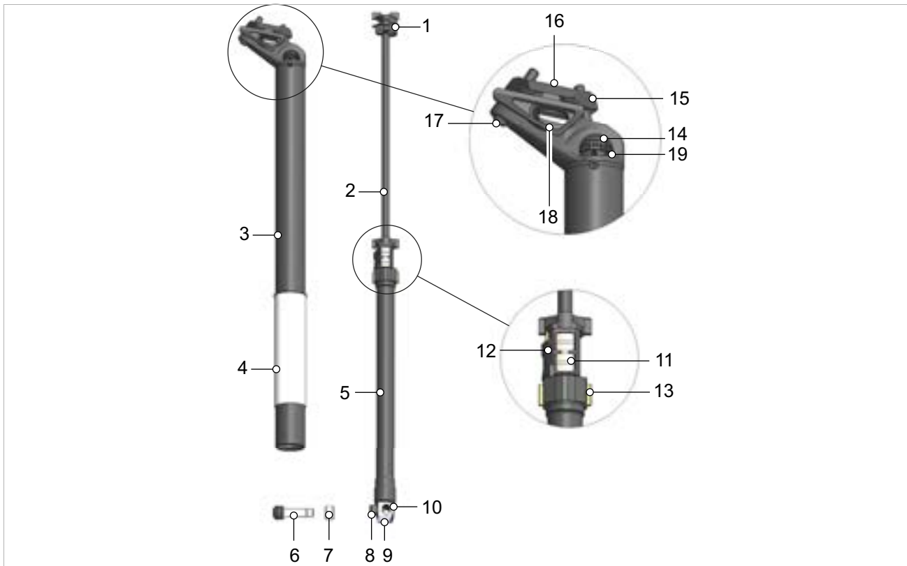
Figure 45: Structure of 8Pins seat post
