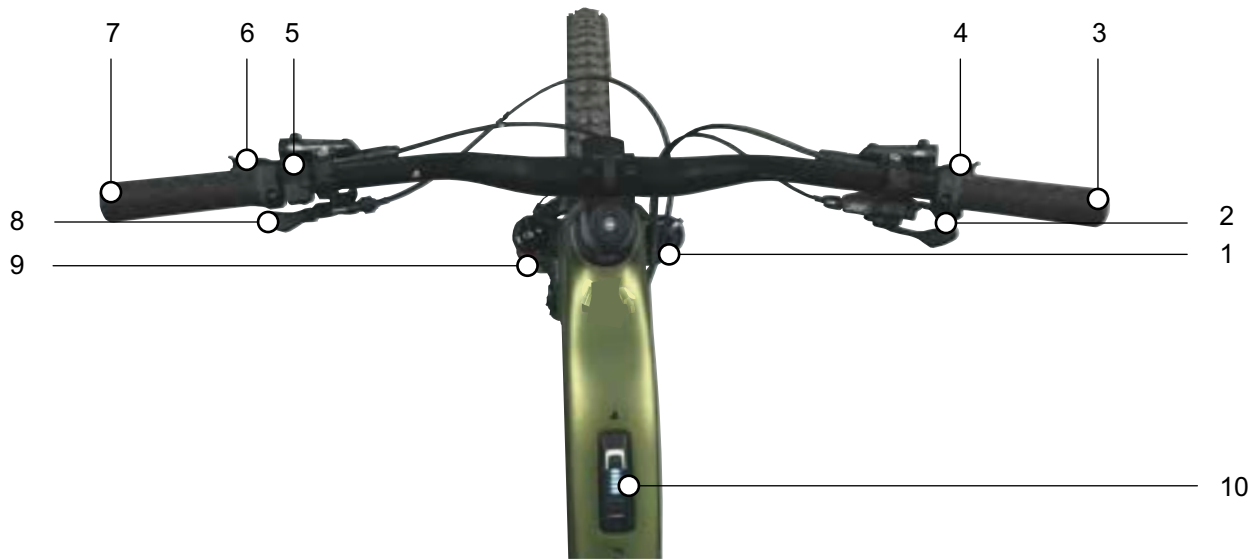
Figure 60: Detailed view of handlebars with BOSCH System Controller on-board computer and Mini Remote – example
