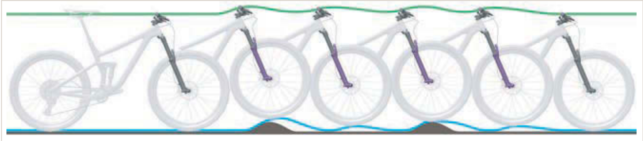
Figure 309: Suspension fork rebounding too quickly
