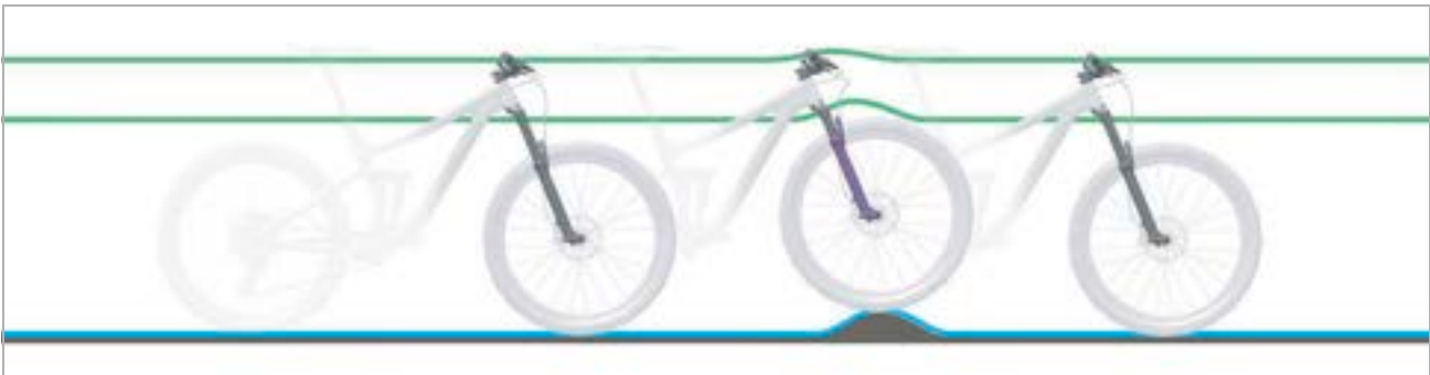
Figure 204: Compression damper set to hard and soft
