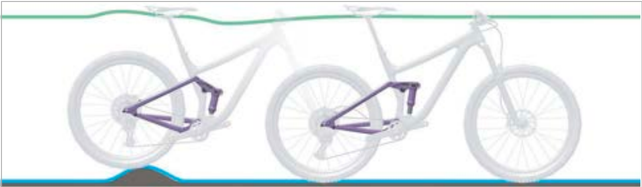
Figure 187: Optimum rear frame damper ride performance over bumps
