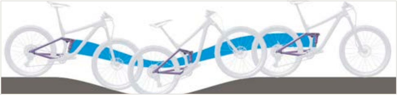
Figure 327: Excessively soft suspension in the rear frame damper on hilly terrain
