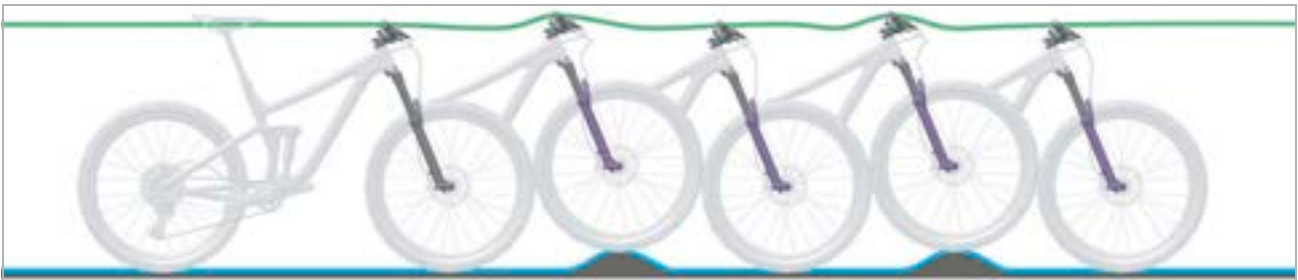
Figure 21: Optimum suspension fork ride performance
