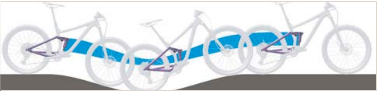
Figure 335: Excessively soft suspension in the rear frame damper on hilly terrain
