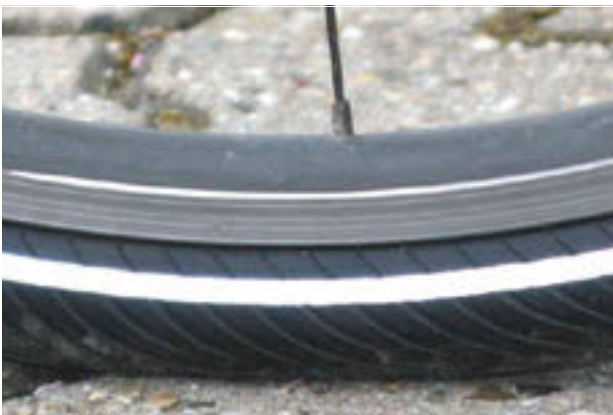
Figure 143: Correct tyre pressure. The tyre is barely deformed under the load of the body weight
