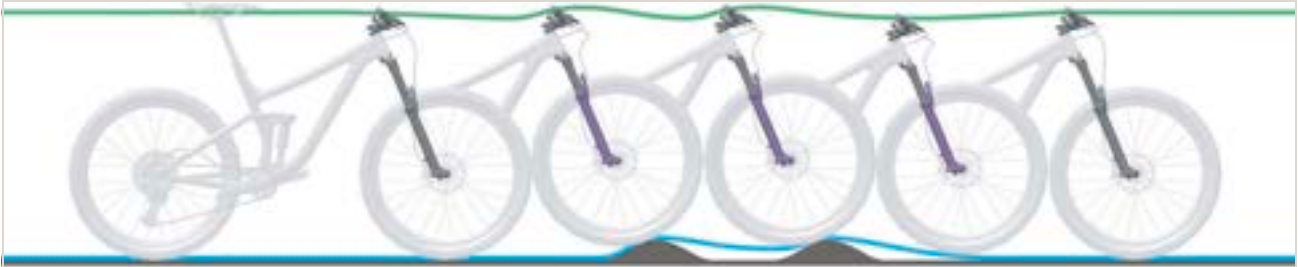
Figure 311: Suspension fork rebounding too slowly
