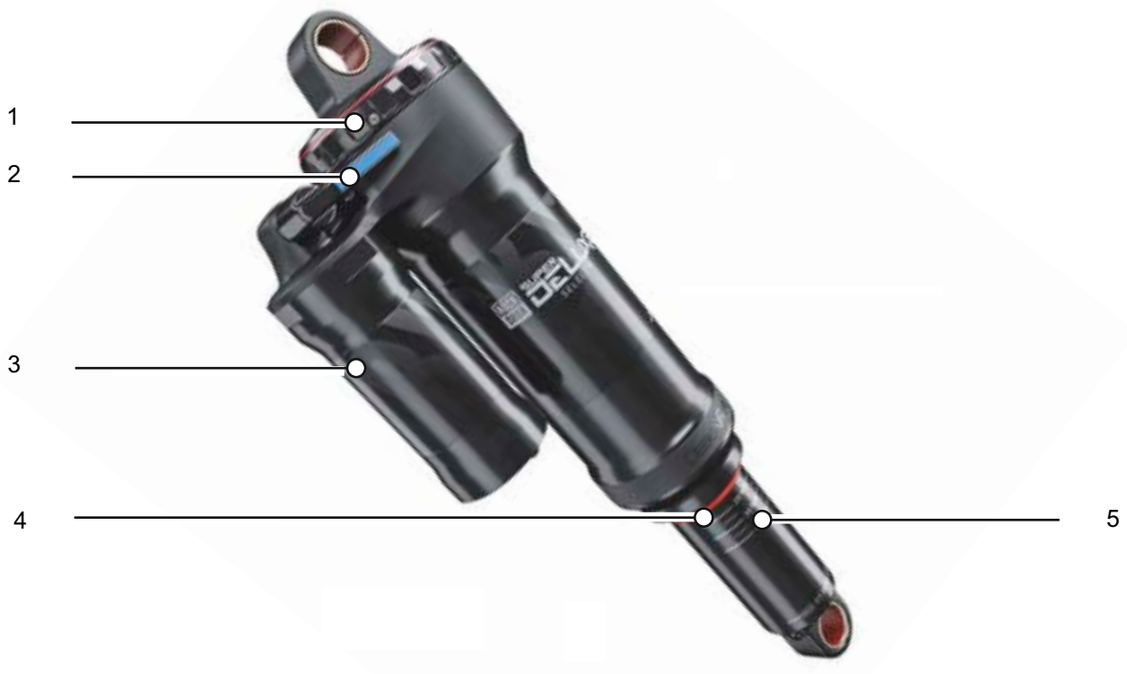
Figure 11: ROCKSHOX Super Deluxe Select+ rear frame damper structure design
