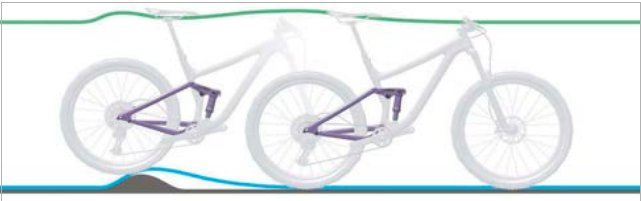
Figure 337: Excessively hard damping in the rear frame damper on bumps
