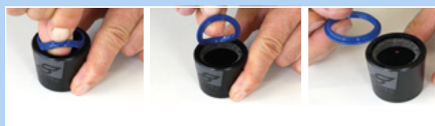
Illustration 140 : Retirer le joint anti-poussière
